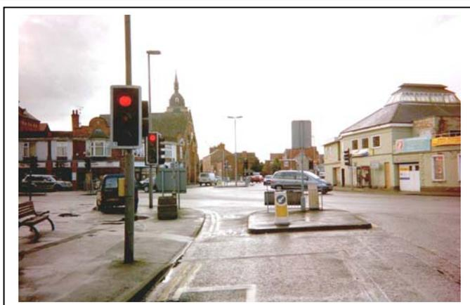
**Photo 6.1** Cycle-only signal control at a junction
